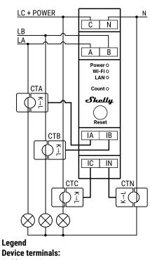
Device terminals: A: Phase A input B: Phase B input C: Phase C and Device power supply input N: Neutral input IA: Phase A current transformer (CTA) input IB: Phase B current transformer (CTB) input IC: Phase C current transformer (CTC) input IN: Neutral current transformer (CTN) input Cables: A: Phase A (110, 240, VAC)
