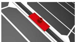
Alternatively: Use two XS middle clamps between two modules
