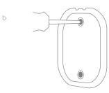
Alternatively, you can use the double adhesive tape to mount the backplate.
