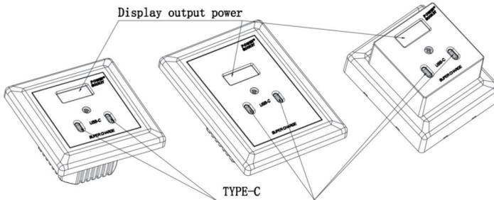
The USB Smart Charging Socket is equipped with an intelligent control chip that can identify the charging modes of different digital devices and automatically switch to the appropriate charging mode. When the device is charging at full speed, the display screen will show the output power in real-time. (The output power is continuously detected within 0.5W within 10 minutes, and the screen will remain bright when charging beyond 4W).
