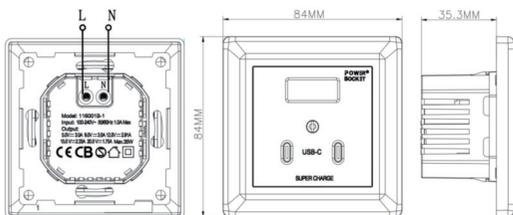
1) The wall USB charging socket can be installed in a standard case with a depth of 40MM or greater.
