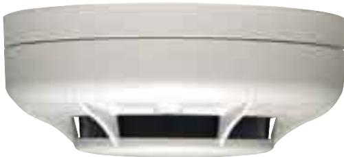
ECO1004 and ECO1005 thermal detectors are available as fixed 58°C and 78°C devices and as rate of rise units. The fixed operating point units are suitable for use in areas where rapid changes of temperature can normally be expected; the rate of rise device in areas where the temperature will normally be relatively stable.
