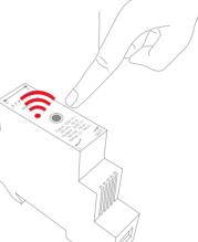
After releasing the button, the red LED will stay on for 2-5 seconds. During that time, the device must not be switched off or unplugged
