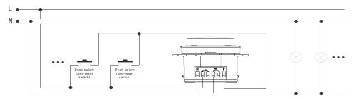
One self-reset switch control multiple dimmers wiring diagram
