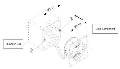
5.4.5 Install the Operation Component to the Fixing Panel and put them together to the Drive Component.
