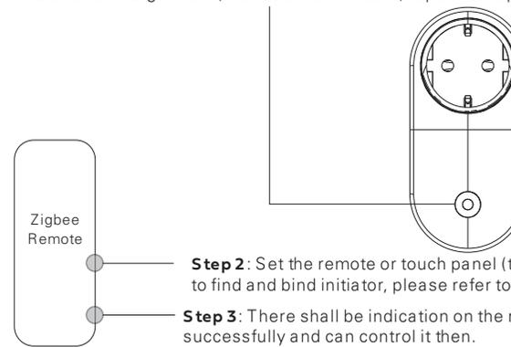
**Step 2:** Set the remote or touch panel (target node) into find and bind mode, and enable it to find and bind initiator, please refer to corresponding remote or touch panel manual.
