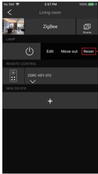
From your ZigBee controller or hub interface, choose to delete or reset the lighting device as instructed. LED indicator of the plug blinks white 3 times to indicate successful reset.
