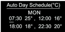
On Auto Day Schedule interface, short press button to select the time or temperature that you would like to modify, then short press move up and down buttons to modify value, then short press button **F** to save and quit, short pressing button only quits without saving.
