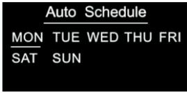
**Schedule setting method 2:** on Home Interface, meanwhile the device is under Auto Mode , short press button to enter into Auto Mode Schedule weekly setting interface quickly:
