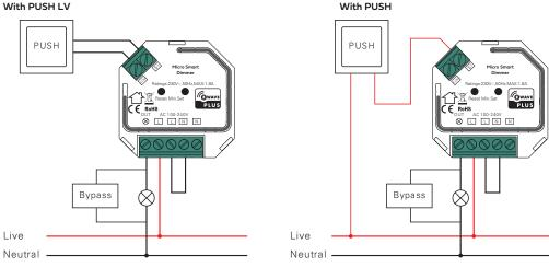
**NOTE:** Switch connected to the S1 terminal activates the basic functionality of the dimmer (turning the light on/off, dimming).
