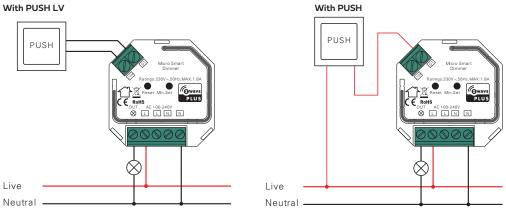
**NOTE:** Switch connected to the S1 terminal activates the basic functionality of the dimmer (turning the light on/off, dimming).
