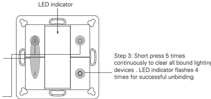
Step 3: Short press 5 times continuously to clear all bound lighting devices. LED indicator flashes 4 times for successful unbinding.
