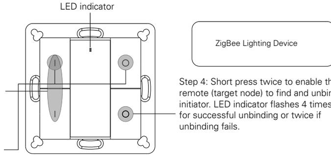
Step 4: Short press twice to enable the remote (target node) to find and unbind initiator. LED indicator flashes 4 times for successful unbinding or twice if unbinding fails.
