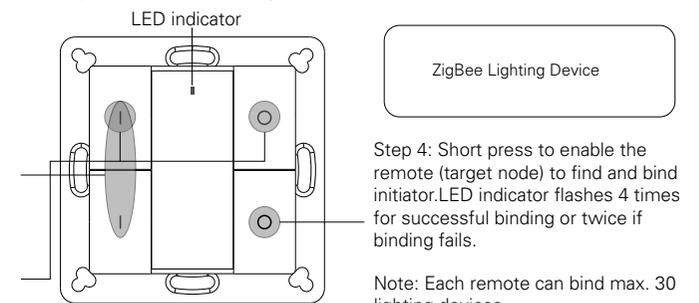
Step 4: Short press to enable the remote (target node) to find and bind initiator. LED indicator flashes 4 times for successful binding or twice if binding fails.
