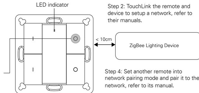
Step 2: TouchLink the remote and device to setup a network, refer to their manuals.
