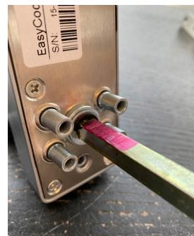
**NOTE! The arrow on the square stick MUST point up and the red mark MUST be up towards the top of the lock, otherwise the lock will not work!**
