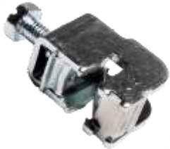
12 004 83 Tilk. Klemme 16-70mm 2 for 5mm kobberskinne
