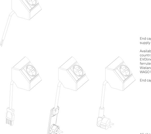
End cap with power input and/or output connector.
