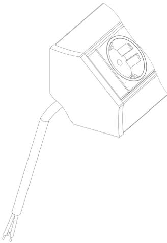
End cap with power input and/or output connector.
