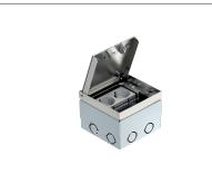
Square flush-mount unit for use in dry-cleaned cavity and screed floors. Fitted plug housing with pre-marked insertion openings for pipes (M25). Cover adjustable to top edge of floor covering using four height-adjustment supports. The minimum installation depth is 95 mm, the height-adjustment range + 20 mm.
