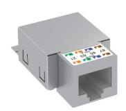
Connection module Cat. 5e shielded, with a RJ 45 slot. Includes an EMC screen hood, a dust cover, a cable tie and mounting instructions. Suitable for installation in data technology supports of type DTG-2RM and DTS-2RM.
