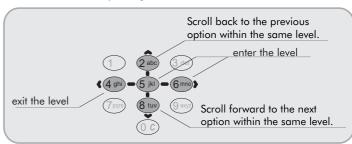
Once you select the desired setting, press the PRG key to store. PRG The entry will begin to flash quickly, indicating that the new setting has been stored
