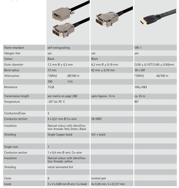
Very high quality cable, that by its construction, transfers the bandwidth (Frequency) of the entire VGA mode. Three 75  $\Omega$  Coaxial cores, the RGB signals with no visible Propagation delays transfered. Six control cores are under others for transmission of the DDC mode and the hardware detect. High transmission quality is ensured by extremely low attenuation structure of the Coaxial cores, combined with a optimal synchronization factor.
