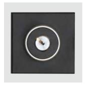
Key with drawal: Position C + A Switch function: Momentary action Switching system: Snap-action switching element Switching capacity: 250 V AC, 5 A
